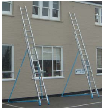
2. STABILISERS IN POSITION
